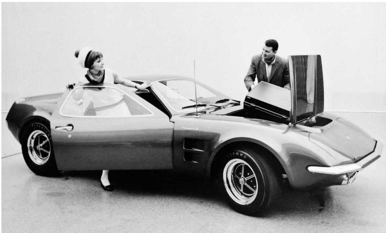
The mid-engine, two-seat Mach 2, which debuted at the 1967 Chicago auto show, relied on various stock Mustang components. Designed by Gene Bordinat and built by Roy Lunn's team, this sporty machine was created under order of Donald Frey as a possible replacement for Carroll Shelby's 427 Cobra.
