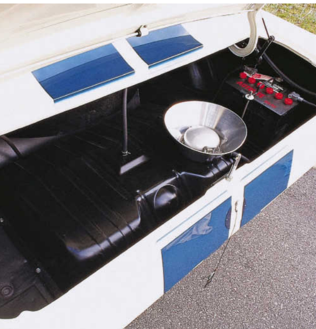
Above: A quick-fill 34-gallon fuel tank went into the R model's trunk, as did the battery and an electric fuel pump. Mike Mueller
