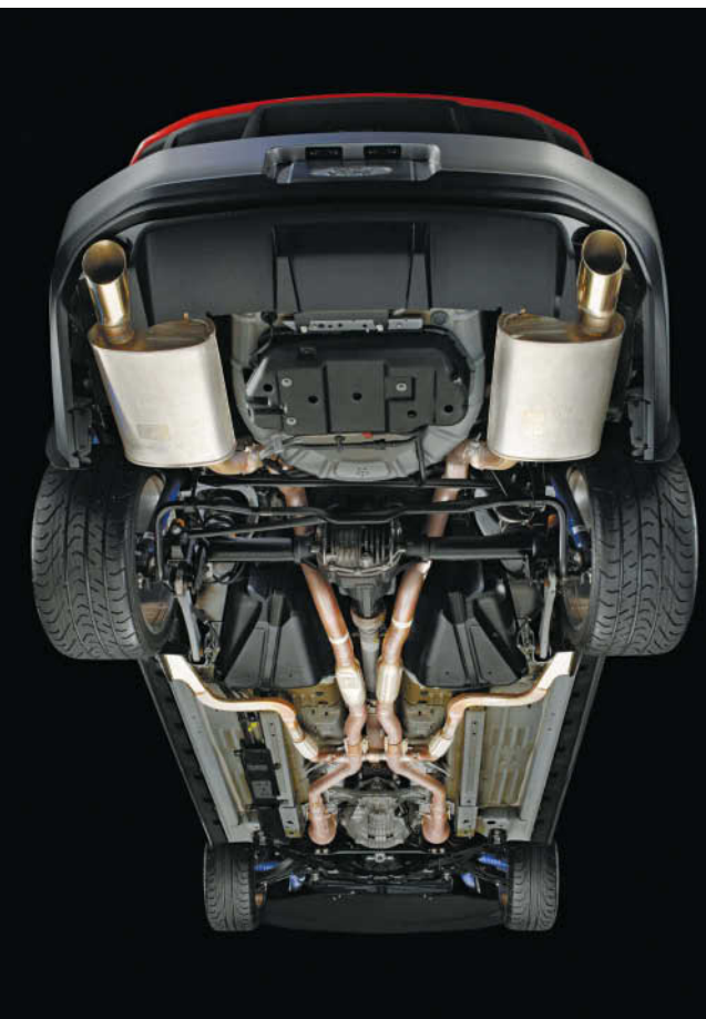
The 2012-13 Boss 302's unique quad exhaust system featured an extra set of tailpipes that exited just in front of the rear wheels—not to improve on the evacuation of spent gases, but to help make this buckin' bronco wail like no other.
