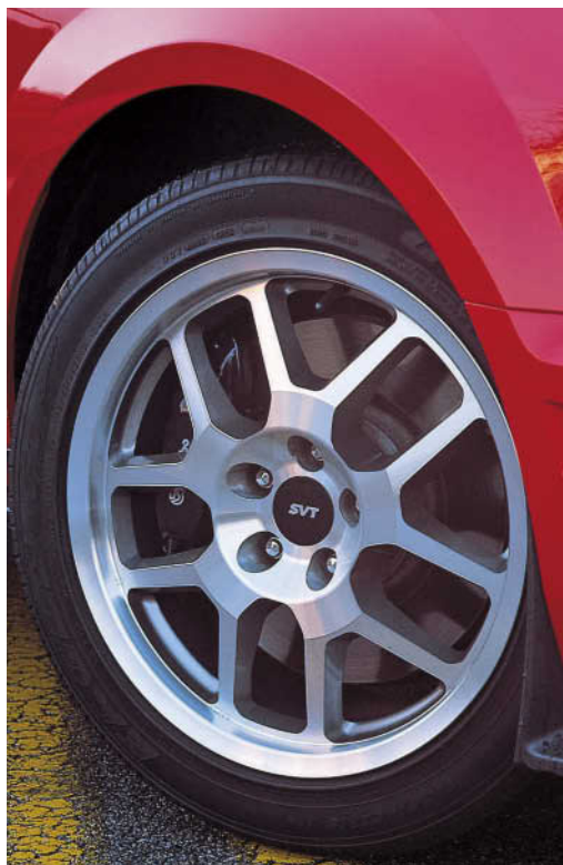
The only exterior SVT identification came in the center of each wheel, which measured 18 inches across and 9.5 inches wide. Tires were P255/45R units in front and P285/40ZR in back. Mike Mueller
