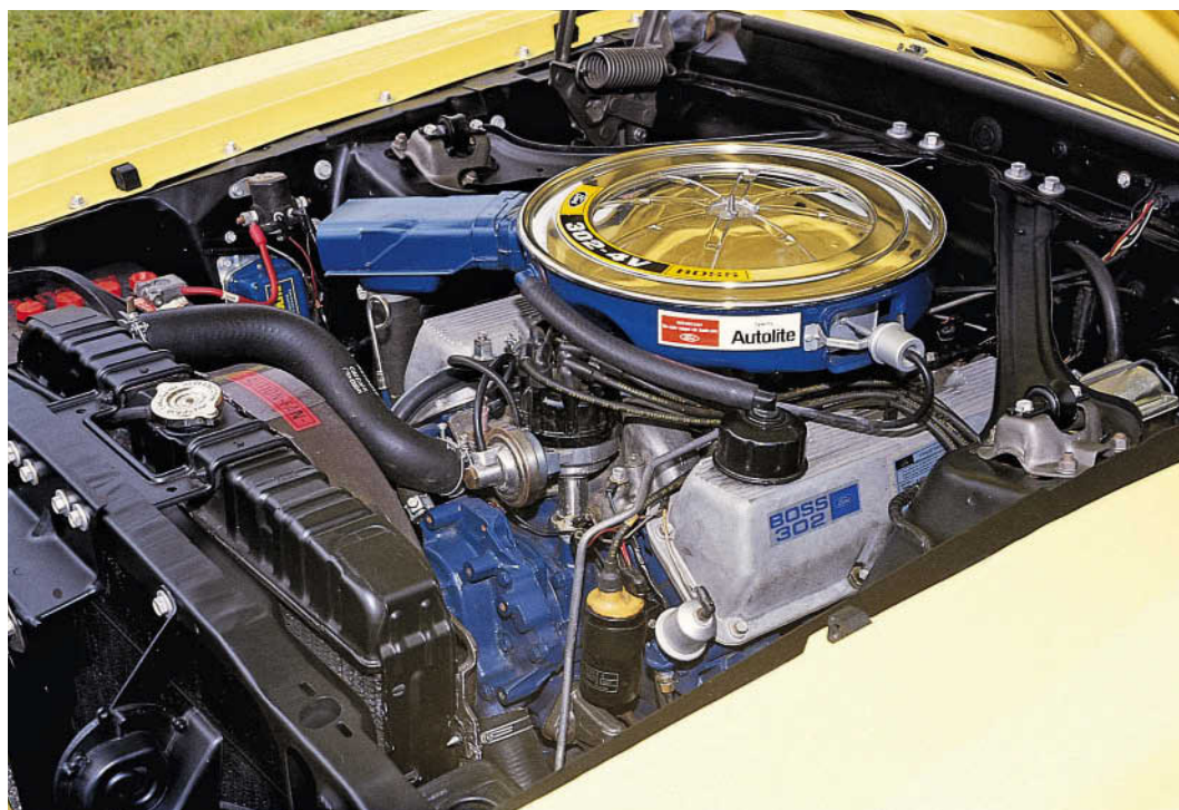
Right: Non-Shaker Boss 302 V-8s in 1970 were topped by a chrome air cleaner lid. Mike Mueller
