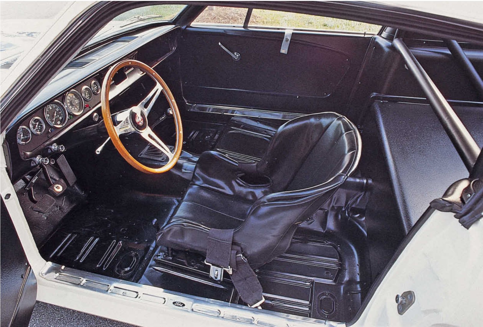
Below: Nonessentials also disappeared inside the GT350R. Carpeting, stock seats and instrumentation, insulation, and the headliner were all deleted. A single bucket seat and four-point roll cage were added. Mike Mueller
