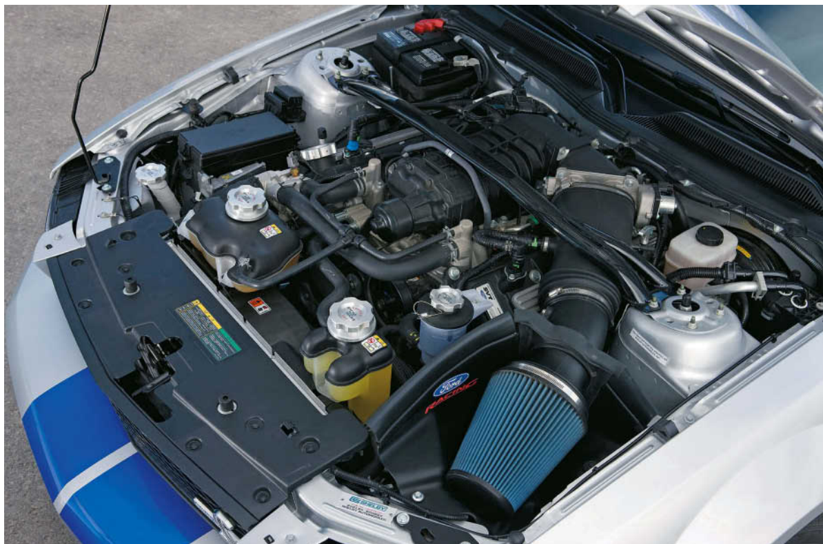
Below: Various Ford Racing power parts helped boost the GT500's supercharged 5.4-liter V-8 from 500 horses to 540 for the new King of the Road Shelby GT500. The 2008 GT500KR was priced at a dizzying $79,995.
