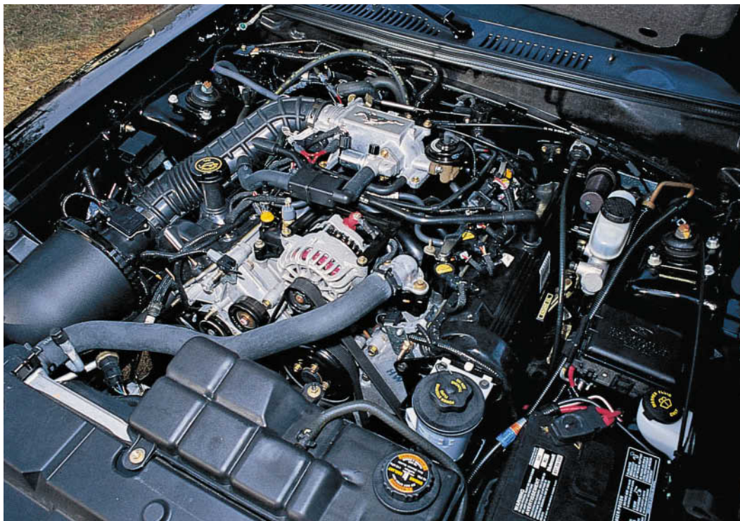
Right: Larger valves, reground camshafts (with higher lift and longer duration), and straightened intake runners helped the GT's 4.6-liter SOHC V-8 make 260 horsepower in 1999. Mike Mueller
