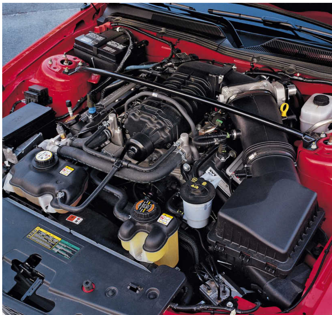
The GT500 came standard with 500 supercharged horses. Producing those horses was a 5.4-liter DOHC Triton V-8 force-fed by an Eaton blower. A six-speed Tremec transmission was standard, too. Mike Mueller
