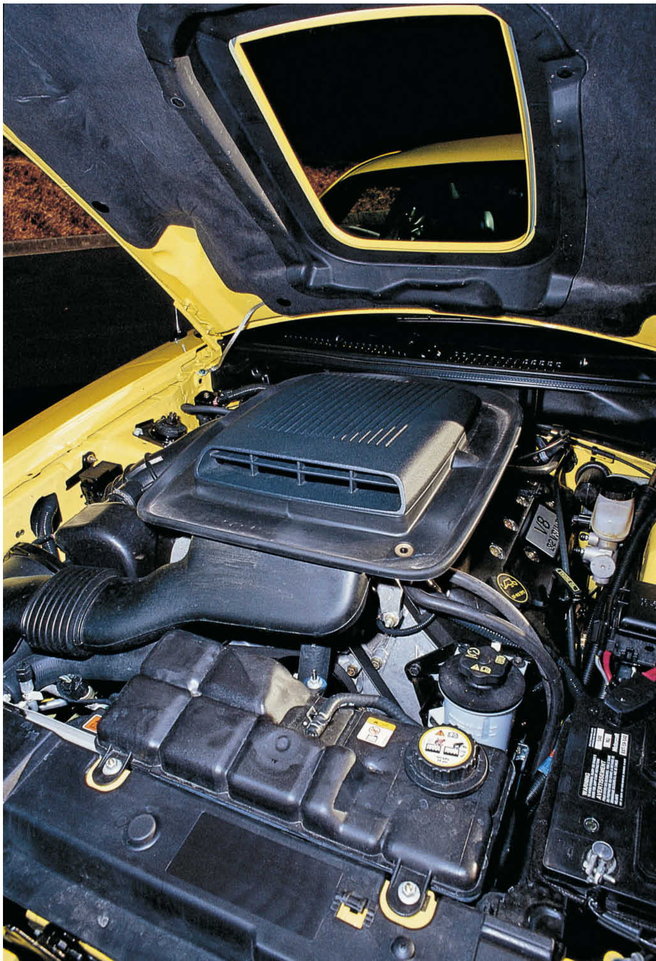
The 2003 Mach 1 was powered by a Cobra-sourced 32-valve DOHC 4.6-liter V-8 topped by yet another retro touch—a Ram-Air Shaker hood scoop. Output for this road rocket was 305 horsepower. Mike Mueller
