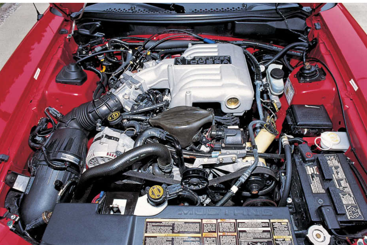
Left: At 240 horsepower, the 1994 Cobra V-8 made 25 more ponies than its 1994 GT counterpart. GT-40 heads with bigger valves helped create that difference. Mike Mueller
