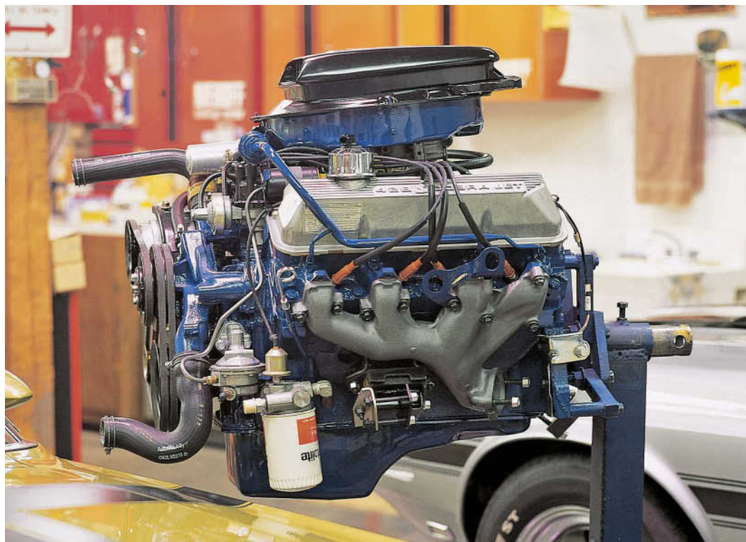
Below: The 428 CJ remained a Mustang option until 1970. The distinctive Shaker Ram-Air system became available atop the Cobra Jet in 1969. Mike Mueller
