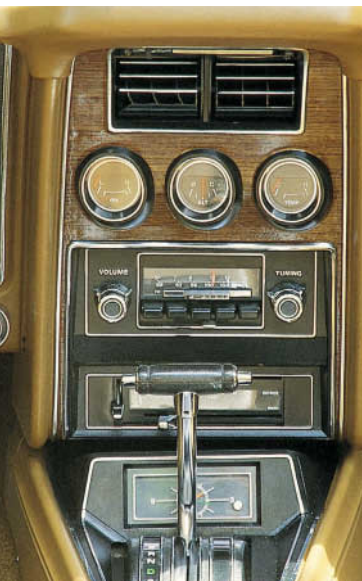
Above: The Instrumentation Group was a $70.83 option for standard Mustangs in 1973. It included gauges for oil pressure, alternator, and coolant temperature. Mike Mueller
