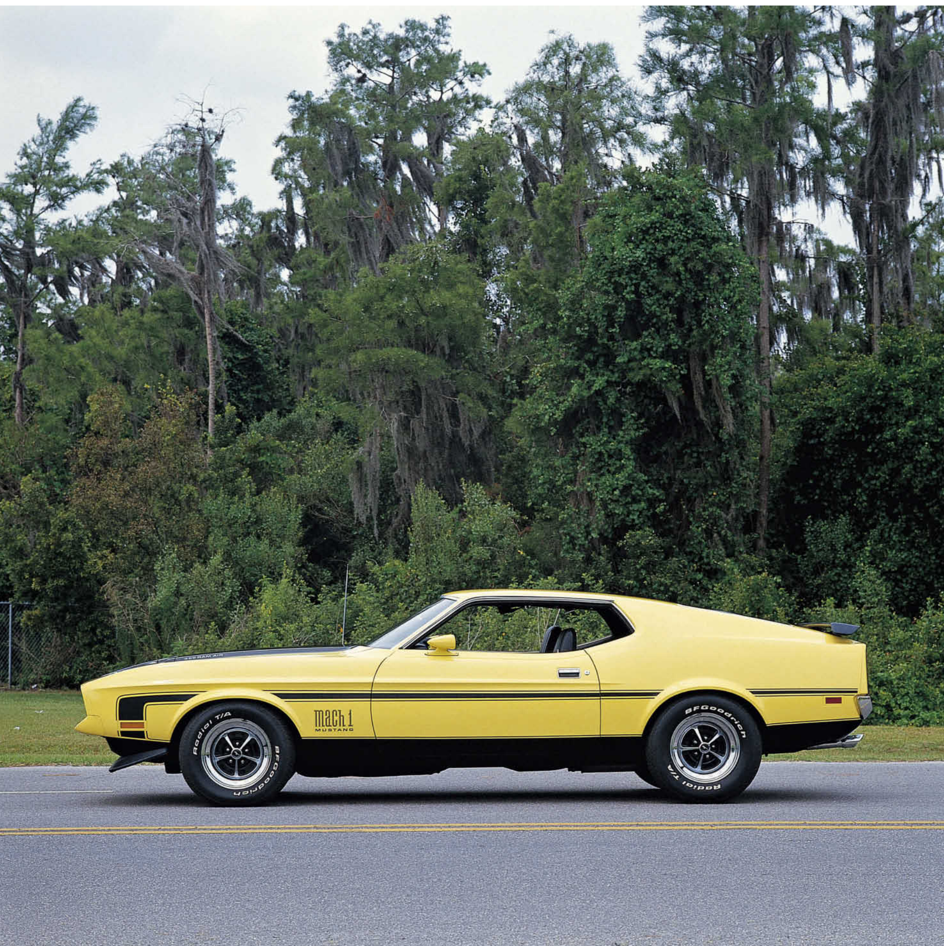
Opposite and above: The supreme Mach 1 for 1971 was fitted with the optional 429 Cobra Jet V-8, which came with or without a functional Ram-Air hood. Mandatory options for the 1971 Cobra Jet Mach 1 included power front disc brakes, Competition Suspension, and fat F70 rubber. F60 Wide Oval tires were optional. Mike Mueller
