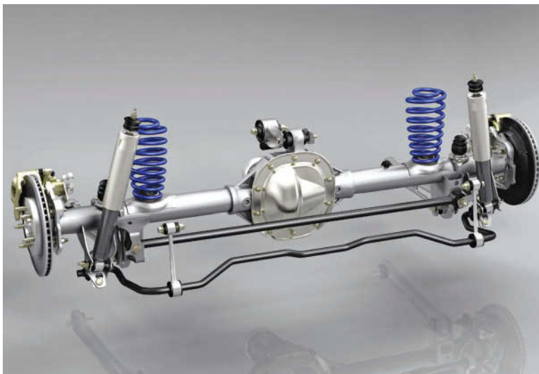
Above: Engineers resisted the temptation to use independent rear suspension (like the SVT Cobra had incorporated from 1999 to 2004) beneath the 2005 Mustang, opting instead to stick with the tried-and-true solid axle in back. A Panhard rod was attached for more precise lateral control of that axle.
