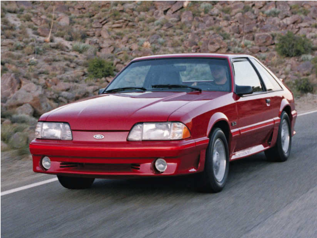
A definitely new aero nose was unveiled for the GT Mustang in 1987, as was some extensive lower-body cladding. New too were the GT's standard 15-inch aluminum wheels in a turbine-style pattern.
