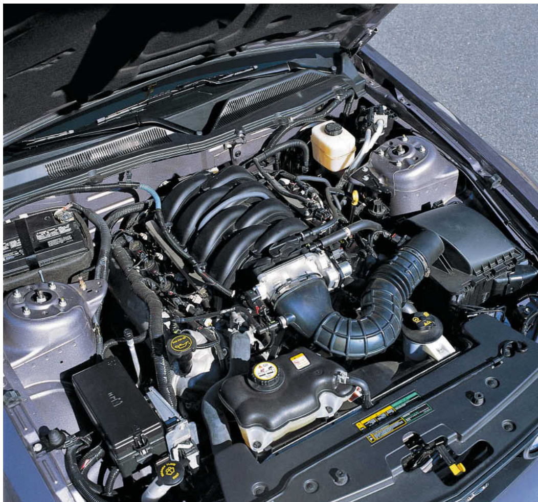
Left: As in 2005, the GT's three-valve, 300-horse V-8 featured variable cam timing and electronic throttle control, both firsts in the pony car field. Mike Mueller
