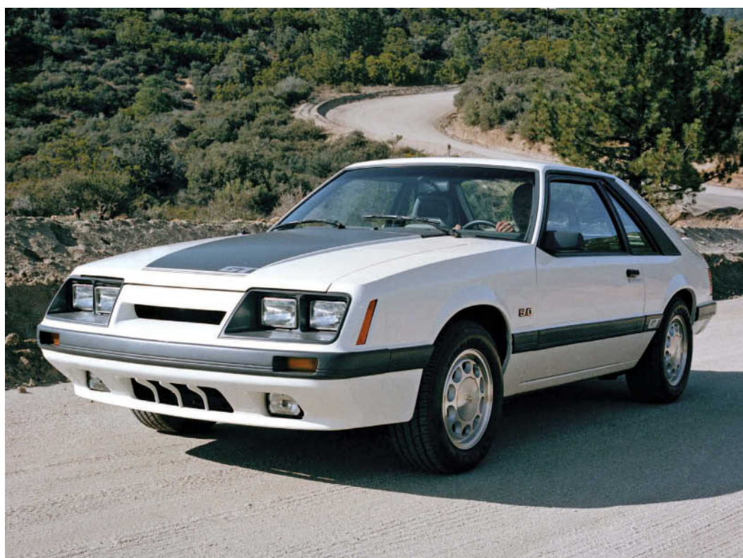
Below: Mustang GTs got new wheels and tires in 1985: Goodyear Eagle P225/60VR Gatorbacks on 15x7 cast-aluminum rims. Output for the GT's HO V-8 that year hit 210 horsepower, a high for the carbureted 5.0-liter.
