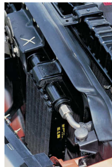
Above: An engine oil cooler was part of the Super Cobra Jet package in 1969 and represented the quickest way to pick one of these mean machines out in a crowd.
