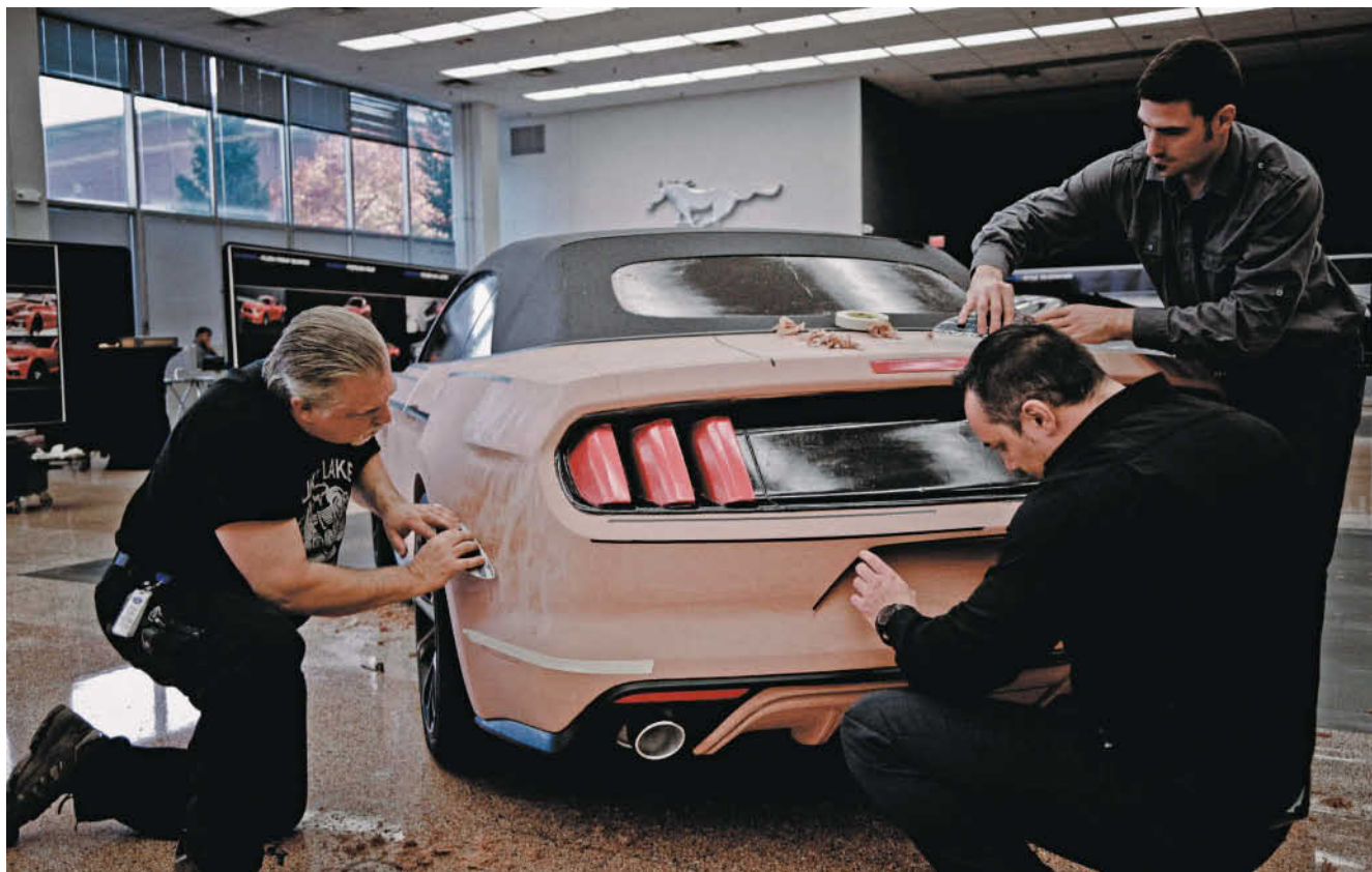
Left: Once sketched on paper, the 2015 Mustang's form typically took shape in full-sized three-dimensional form using sculpted clay.
