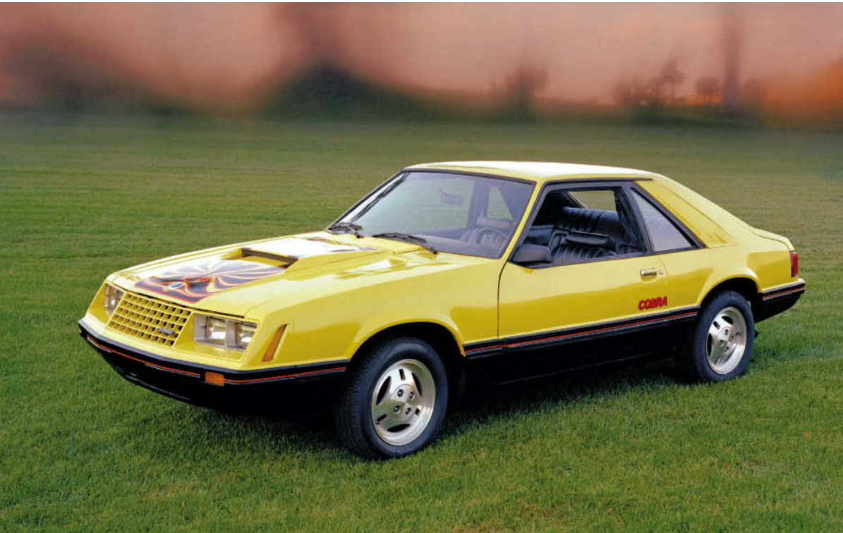
Along with its splashy graphics, the Cobra package for 1979 included a tuned suspension with Michelin metric TRX tires on forged-aluminum wheels. The 2.3-liter turbocharged four-cylinder was standard; the 5.0-liter V-8 was a no-cost option.
