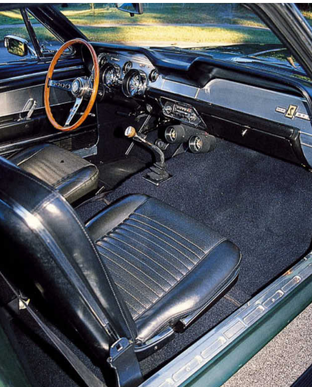
Above: A wood-rimmed steering wheel, 140-mile-per-hour speedometer, and 8,000-rpm tachometer were standard inside the 1967 Shelby Mustang, as was a special underdash housing containing amp and oil pressure gauges. Mike Mueller
