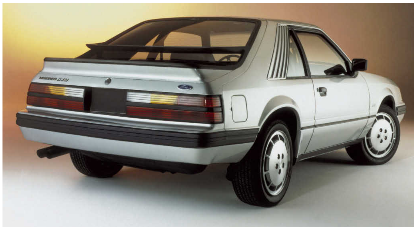
Left: Wearing an eye-catching biplane spoiler, the 1984 SVO Mustang was equally unconventional in back. Body cladding was also standard just ahead of the rear wheels.
