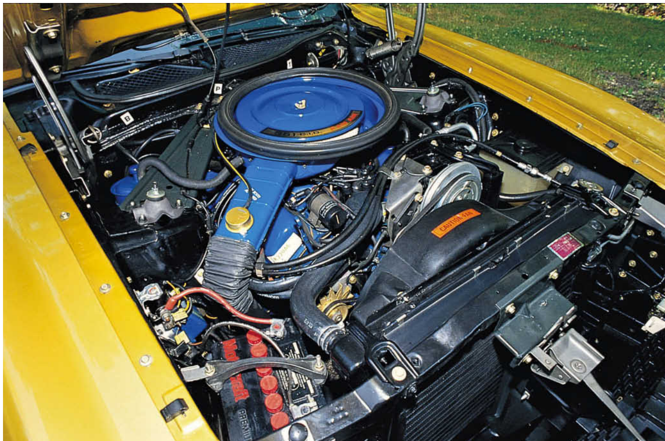
Right: Priced at $40.79, this optional 351 Cleveland two-barrel V-8 was rated at 177 horsepower in 1973. The Dual Ram Induction hood cost $76.33 that year. Mike Mueller
