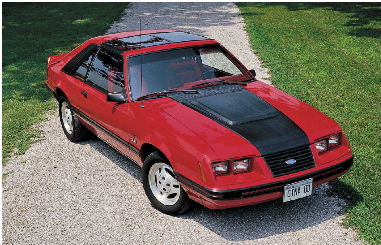
Left: GT Mustangs were available in 1983 with either the 5.0-liter HO or revived turbocharged four-cylinder. This T-top GT features the HO V-8, uprated to 175 horsepower for 1983. Mike Mueller
