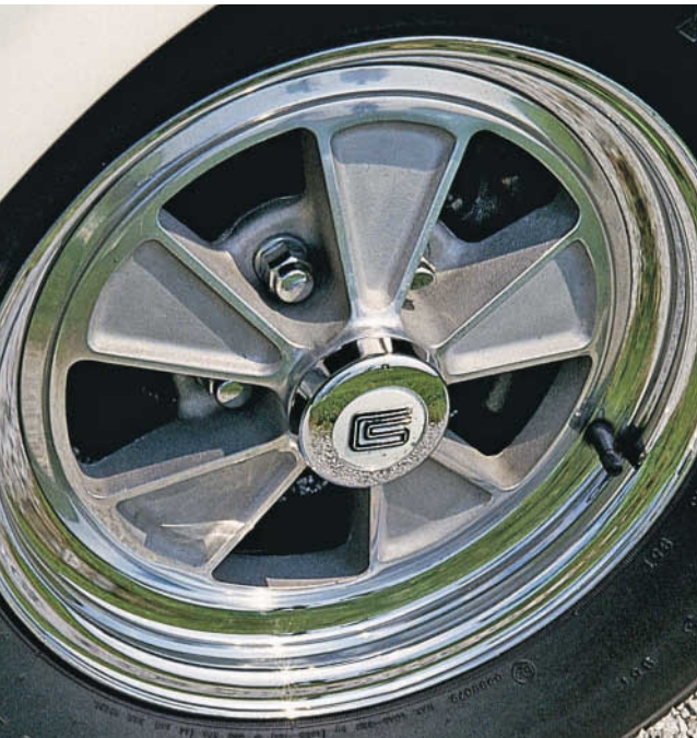
Below: Early 1966 Shelbys were fitted with these 15-inch five-spoke Cragar mag wheels. Later models that year got 14-inch Magnum 500 rims. Mike Mueller
