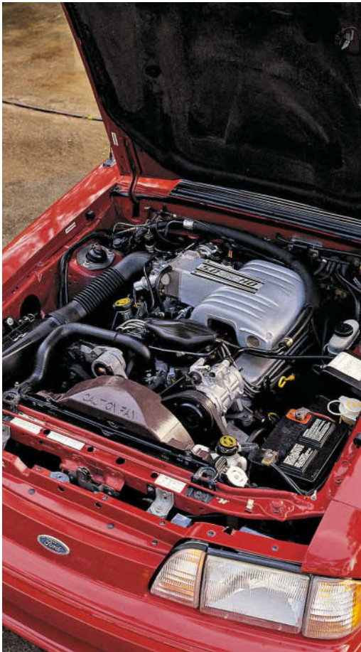
The 225-horsepower HO V-8 made hay on the street scene from 1987 to 1992. Roller lifters and tubular headers helped this hot little small-block handle anything a Camaro driver could throw at it. Mike Mueller
