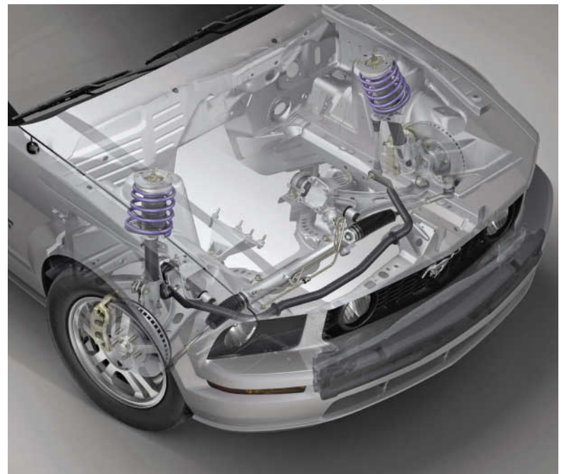
Right: MacPherson struts continued to be the norm up front but were now bolted up on the bottom end to lightweight-yet-thoroughly-stiff reverse-L control arms. Rack-and-pinion steering carried over from 2004.
