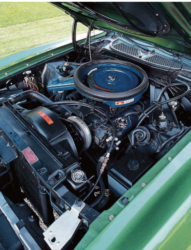
Above: A 302 two-barrel V-8 was again standard for the 1972 Mach 1. The 351 Cleveland two-barrel (shown here) was optional. The Dual Ram Induction hood was available only with this engine in 1972. Four-barrel 351s came with a nonfunctional NASA hood. Mike Mueller
