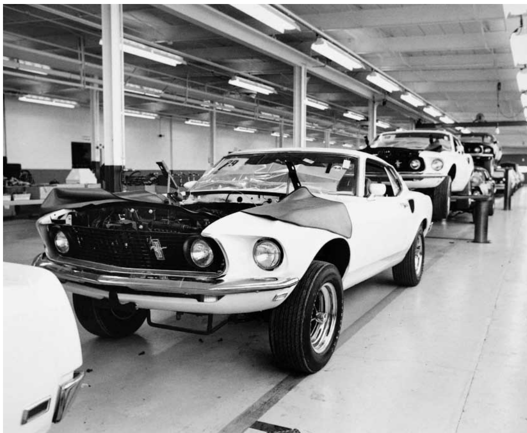
Above: The big Boss 429 V-8 was literally shoehorned between Mustang flanks at the Kar Kraft works in Brighton, Michigan.
