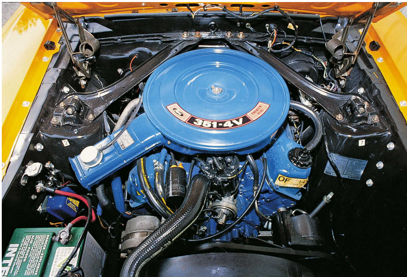
Above: A 351 two-barrel V-8 was again standard for the Mach 1 in 1970. Shown here is the optional four-barrel 351 Cleveland small-block, rated at 300 horsepower. Mike Mueller
