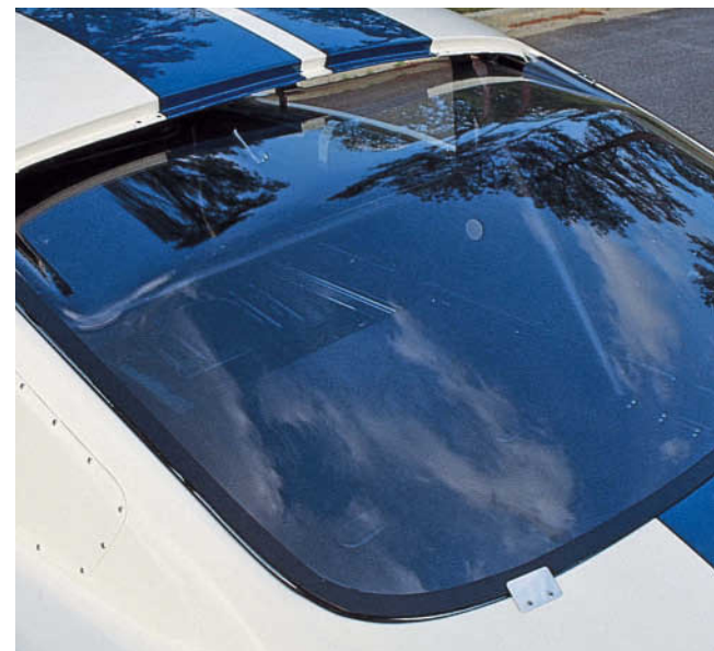
Above: The R model's weight-saving Plexiglas window shaved off some 20 pounds in back. Mike Mueller
