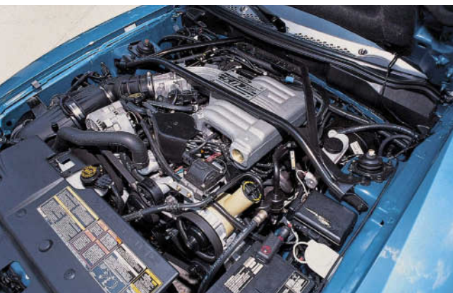
There was no skimping beneath the 1995 GTS coupe's hood. The GT's 215-horse HO V-8 carried over untouched. Mike Mueller
